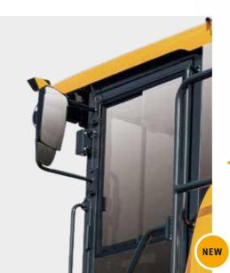
Foldable side mirror The side mirror is easy to adjust for optimal visibility and can be folded away to prevent damage during transportation.
