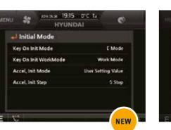
Key On Init Work Mode This feature allows operators to save the attachment mode setting so that the machine is automatically in the right work mode when re-starting.
