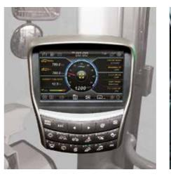
Wide touchscreen monitor The HX260AL features an 8-inch display with a touchscreen and excellent legibility. All the indicators displaying machine status are centralised in one cluster to enable easy, efficient control.
